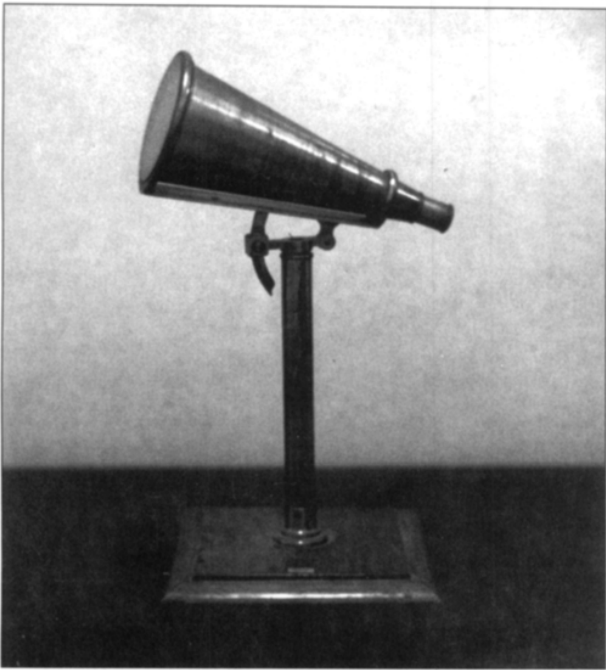
Fig. 6 Wheatstone precision polarization sundial, by W.H. Darker of Lambeth. The cone is 25 cm long. (Wellcome Collection, Science Museum, London.)
