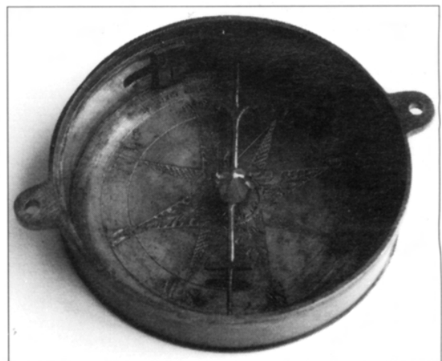
FIGURE 9: Adjustable 'North' marker in the compass bowl of a dial by Thomas Heath, London. Its position may be moved from outside the compass bowl
