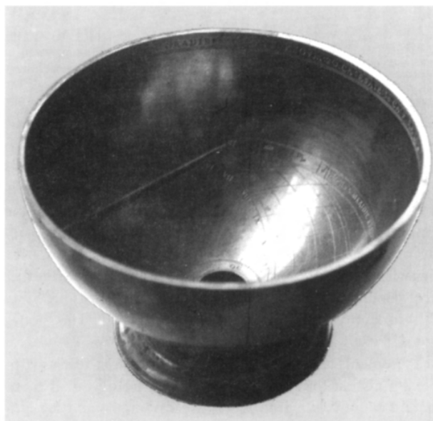
Figure 5: Refractive equal-hour scaphe by Georg Hartmann of Nuremberg, dated 1547. Courtesy of the Museo de Santa Cruz de Toledo, Spain. Inventory No.286.
