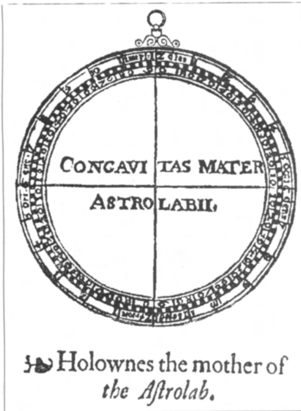
FIGURE 3: The Mater , a shallow round box with a slightly elevated, graduated rim.
