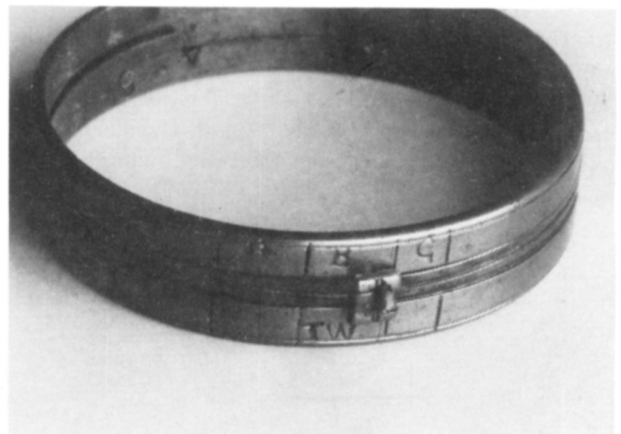
FIGURE 3: Poke Dial by T.W., showing the three bands A, B & C. It clearly shows the irregularities of the Punch Markings.
