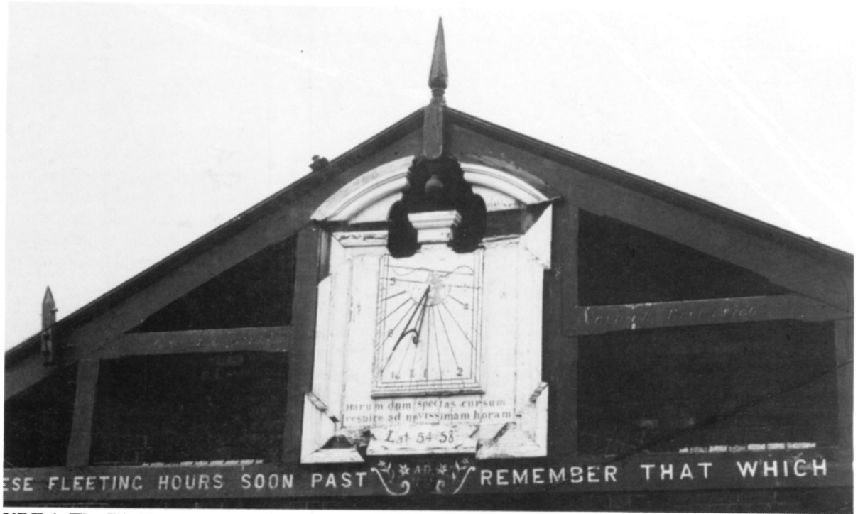
FIGURE 1: The Dial in place at the entrance to the Neptune Shipyard. On the centre beam is carved “Walker is 6 minutes behind Greenwich”.
