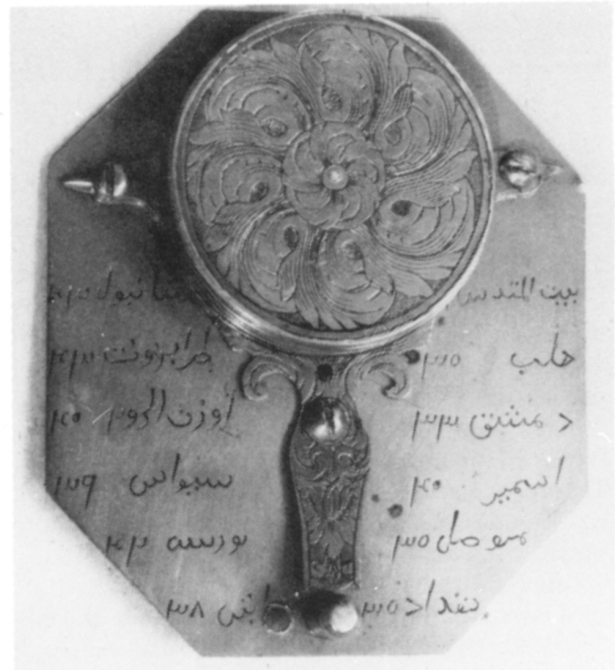
FIGURE 4: 'Butterfield' style dial by Le Maire et Fils, brass, circa 1730. Made for the Arabic market with a list of towns and their latitudes.
