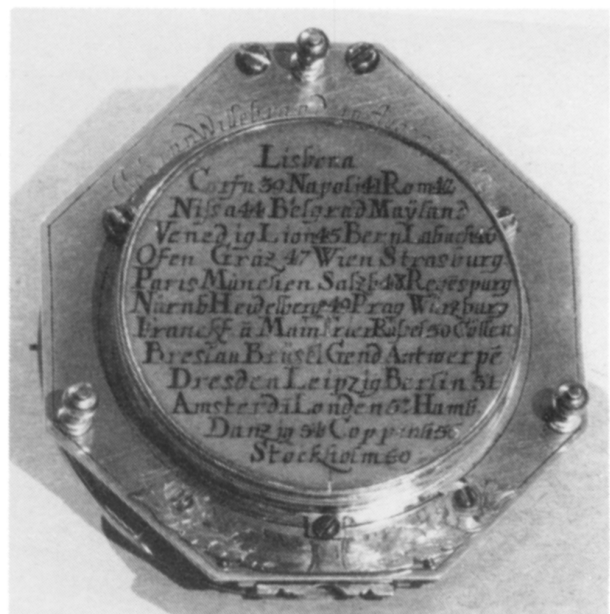
FIGURE 2: Augsburg dial signed Johannes Willebrand, of silver and gilt metal, with list of European towns with their latitudes, circa 1700.
