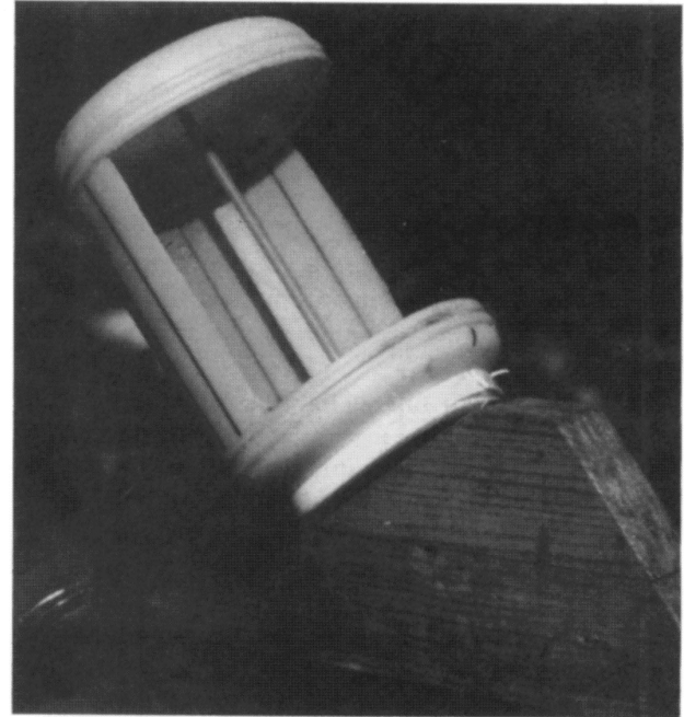
Fig 2. Novel Translucent Sundial (Viewed from Front)
