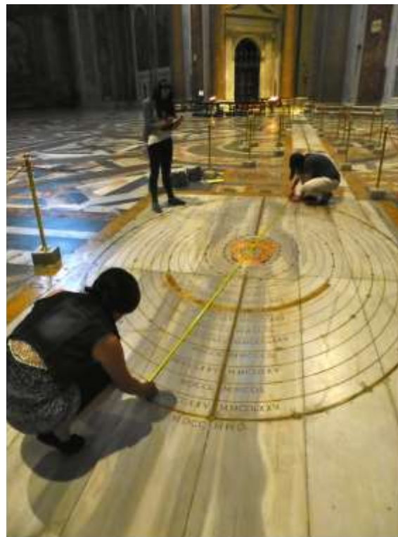
Fig. 19. Measuring the dimensions of the precession ellipses (looking north). Note that their major axes run 0.91 metres to the west of the meridian line. Photo: Sullivan.
