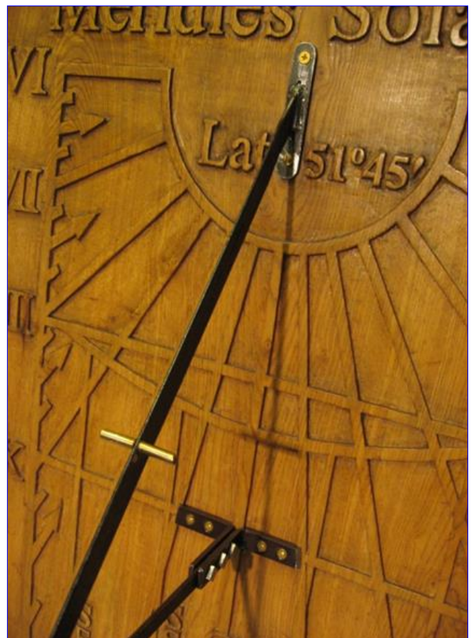
Fig. 10. Close-up of the new dial, with linseed oil applied and showing the gnomon fixing and the brass nodus.
