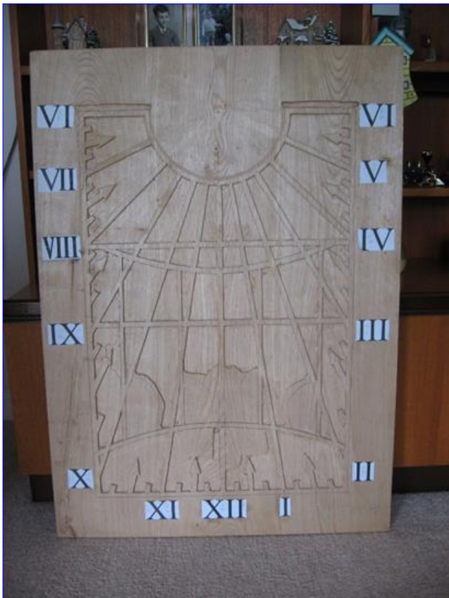
Fig. 8. The new dial with some areas still to be removed by the router.
