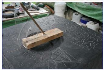
Fig. 7. Setting the gnomon for the St Andrews University Museum Sundial: first, the bronze rod was set in the wax original to form the gnomon and then, after incorporating the gnomon in the mould, preserving its position exactly, the cast was made round the gnomon, replicating its position in the final result.
